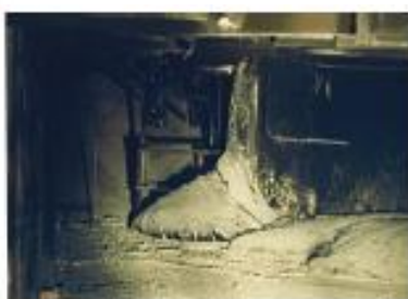
Photograph B Fuel debris of Chernobyl
