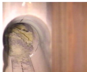
Photograph C Fuel debris of Fuel debris of Windscale
