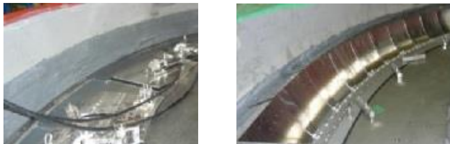
Element tests conducted on seal inside the RVP
