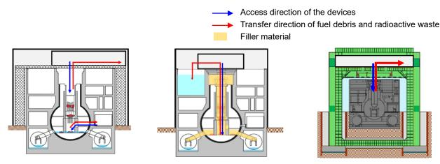
(a-1) Partial submersion method (a-2) Partial submersion method option (water injection into RPV) (RPV filling and solidification)
