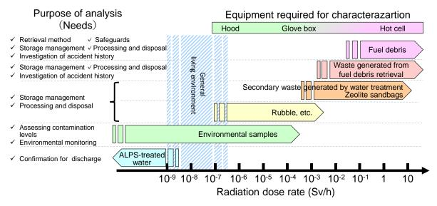
Fig. 11 Relationship between the purpose of the analysis, equipment required for characterization, and radiation dose rates of the analysis targets
