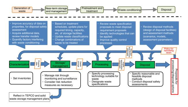
Fig. 7 Procedure to reasonably select safe processing/disposal methods of solid waste
