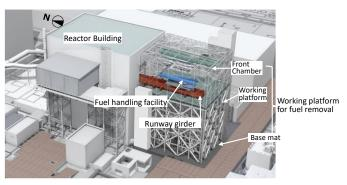
Fig. 10 Fuel removal method in Unit 2 SFP
